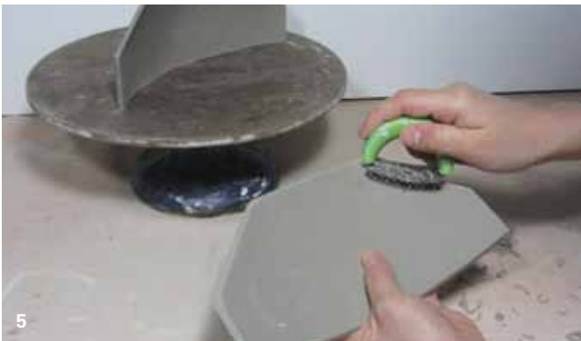
5 Use a rasp to create a 45° bevel on the edges of the two pieces. Score and slip the edges of the piece.
