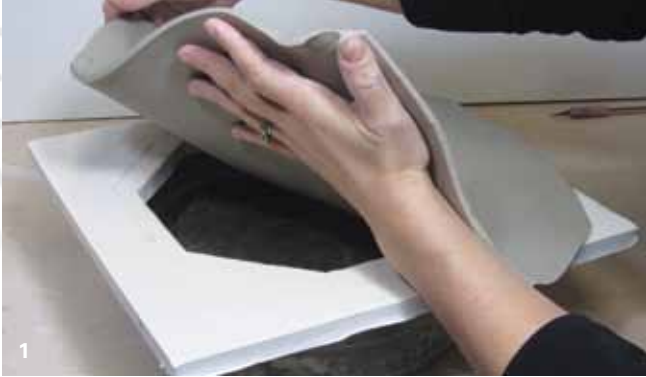
1 Cut out an octagonal template. With the template supported, drape a slab onto the mold.
